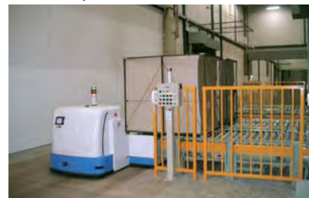
● The cargo is shifting from AGV to feeding conveyor in a deliver area.
