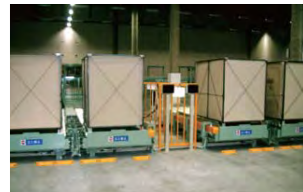
● Station conveyor (Products weight 1,000 kg/1pc)
