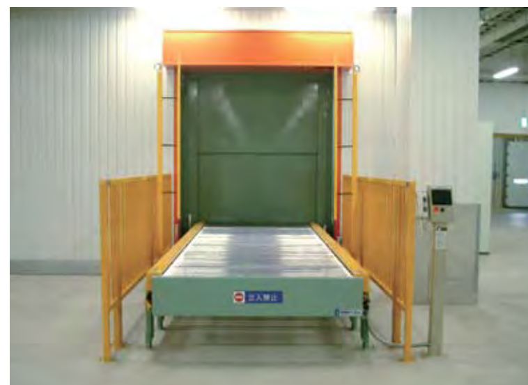
● Newly installed Omni-Lifter after removal of elevator (NEDO target goods)
