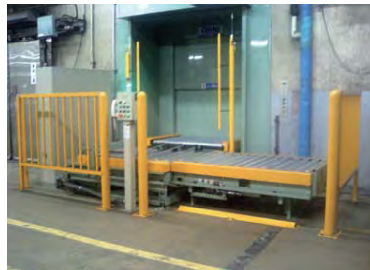
● Newly installed Omni-Lifter after removal of elevator (NEDO target goods)
