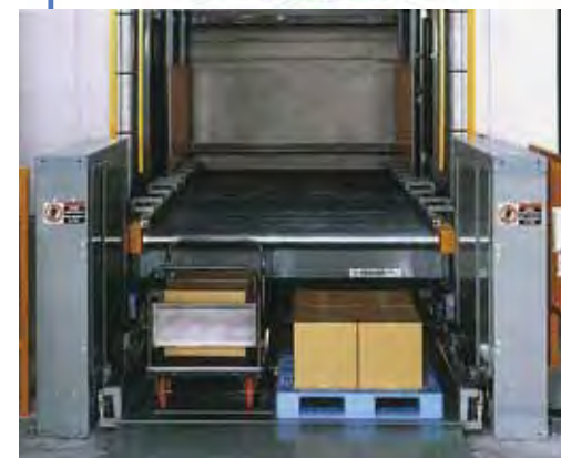
● It is possible to transport a pallet and a trolley at the same time.
