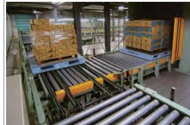
● Change in direction of pallet on the conveyor will be done by chain up-down device.
